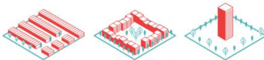
Picture 1. – Sites with the same housing units density and different typology of buildings [10]
